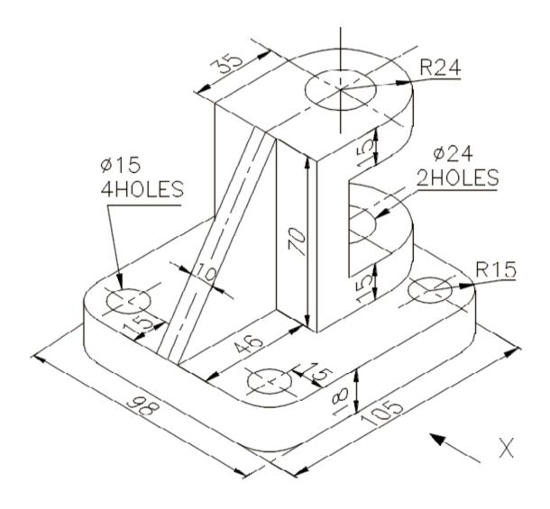
Draw by using 1st **OR** 3rd angle method of projection i) F.V, ii) T.V. & iii) R.H.S.V
