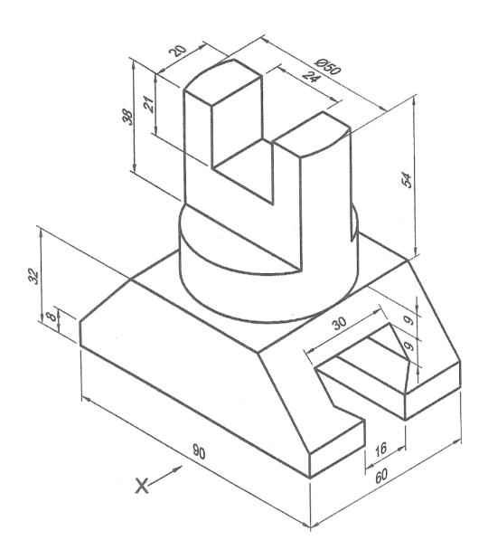
Draw by using  $1^{st}$  **OR**  $3^{rd}$  angle method of projection i) F.V, ii) T.V. & iii) L.H.S.V
