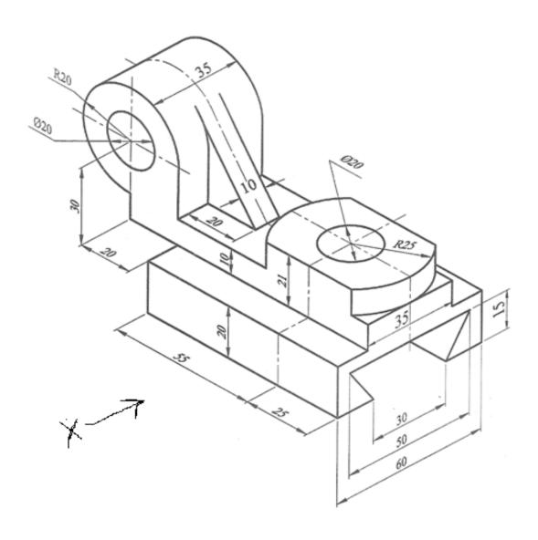
Draw by using  $1^{st}$  **OR**  $3^{rd}$  angle method of projection i) F.V, ii) T.V. & iii) L.H.S.V
